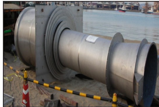
The telescoping granulated slag chute at discharge pier in steel mill
